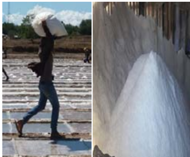
Fig. 23. Storing of salt in kamalig for further drying.
