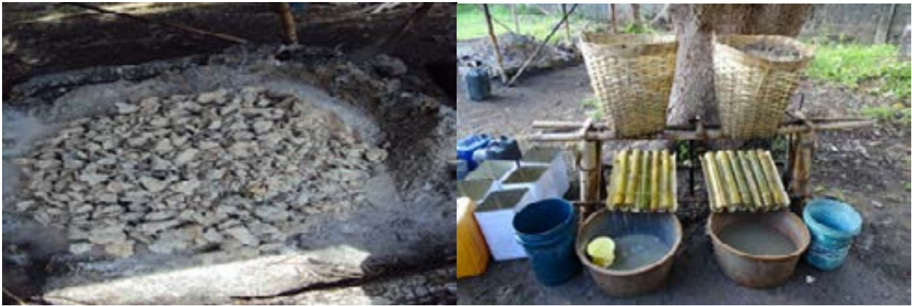
Fig. 17. The process of collecting ashes poured with saltwater to cool it down (left) and gathering of cooled ashes in two large kaings which is placed in elevated form (right).
