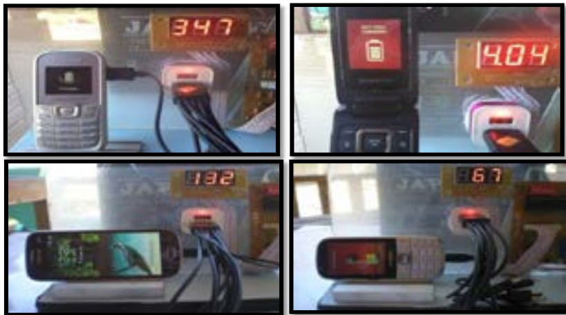
Figure 20. Charging and compatibility test of the system using the generic mobile phone brand.
