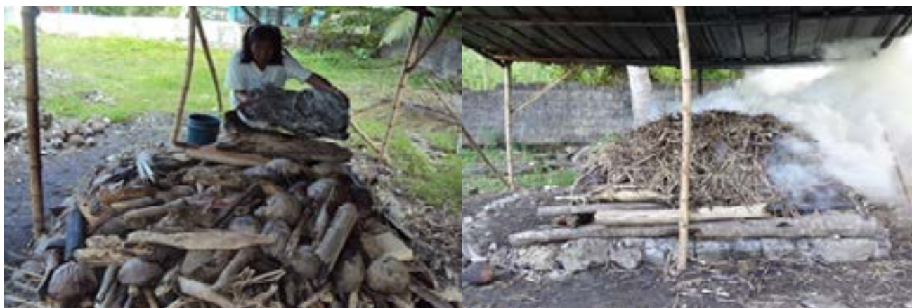
Fig. 16. Piling of bambooes and woods for firing process of making Tultul
