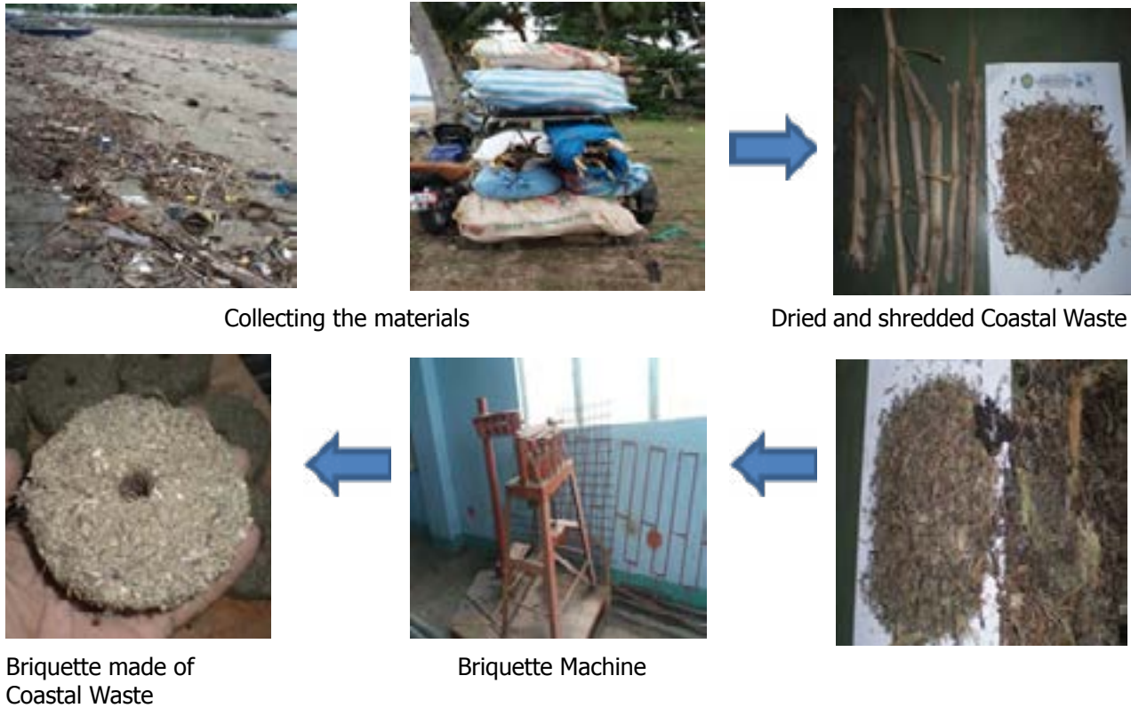
Figure 1. Production of Briquette from Coastal Waste
