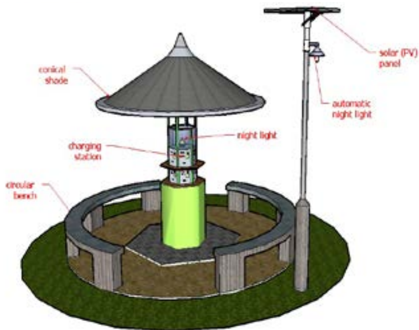
Figure 1. Detailed design concept and perspective of the solar-powered coin-operated charging station
